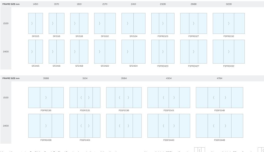
Viewed from exterior: S = Sliding Panel, F = Fixed Panel Arrow indicates sliding direction
