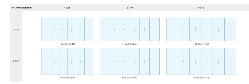
Viewed from exterior: **S** = Sliding Panel, **F** = Fixed Panel Arrow indicates sliding direction
