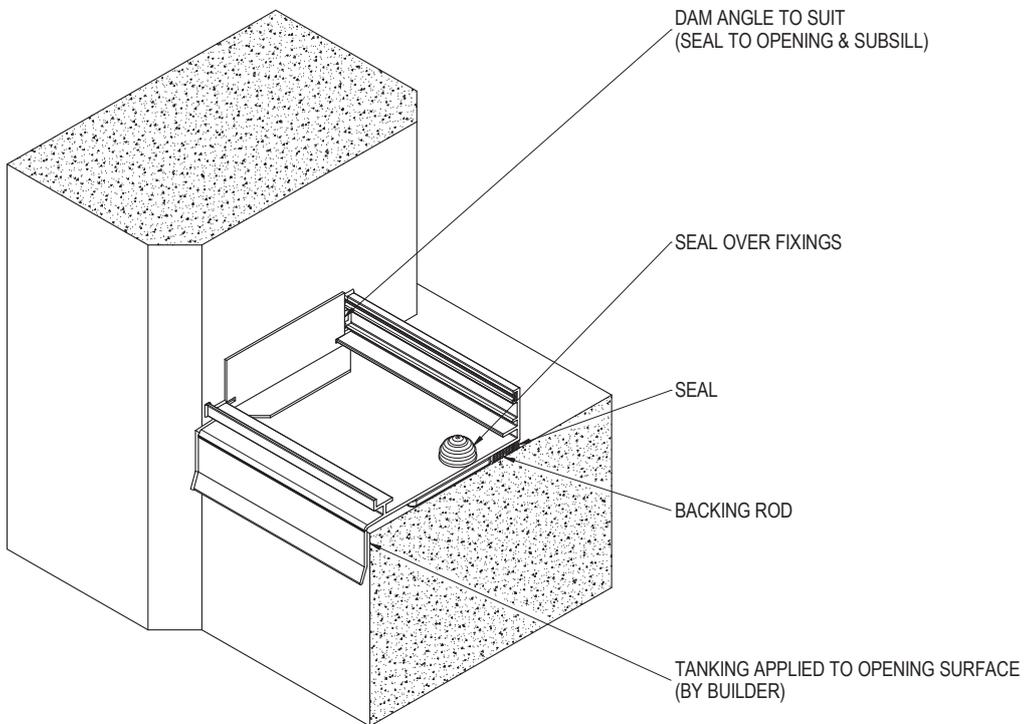
2. APPLY SEALANT TO VERTICAL FACE OF DAM ANGLE AND ALSO TO THE FLOOR OF THE SUBSILL. POSITION DAM ANGLE AGAINST STRUCTURE. SEAL ALL JOINTS BETWEEN ANGLE AND SUBSILL. SEAL ALL JOINTS BETWEEN ANGLE AND SUBSILL. SEAL OVER FIXINGS AND UNDER SUB SILL TO STRUCTURE.
